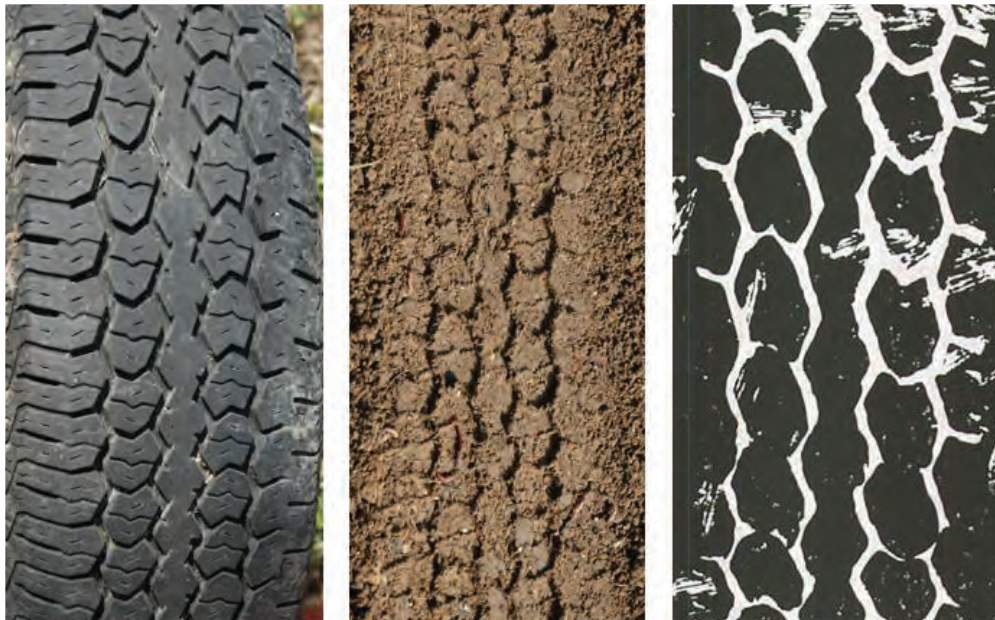
Figure 15.37 Tire tread; (l-r) tire, impression, imprint
