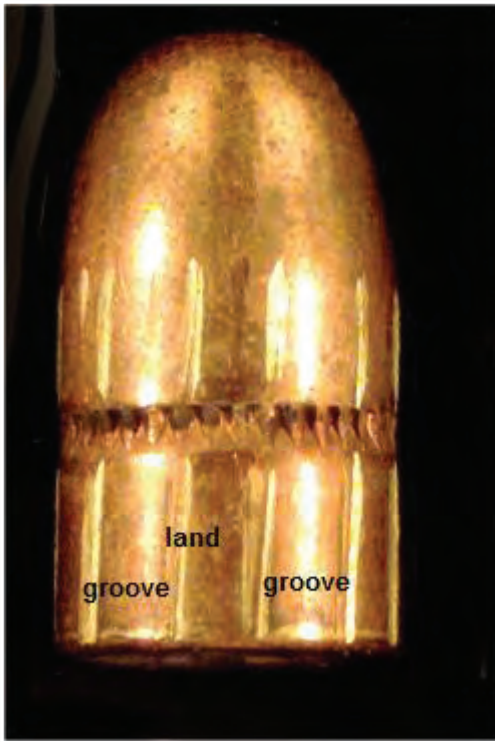
Figure 15.9 Right-twist lands and grooves in brass-clad bullet
