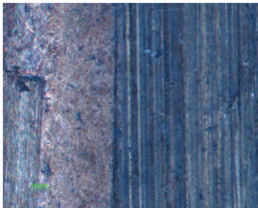
Figure 15.10 Striae on .38-caliber copper-clad bullet
