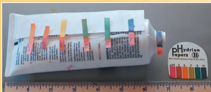
Change in pH from bottom to top of “unknown” hair conditioner tube
